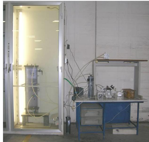
*Anaerobic Membrane Bioreactor (Progetto Aquafit 4use)*
